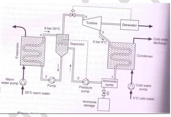
A closed cycle OTEC system is shown in figure. It contains the following parts.
